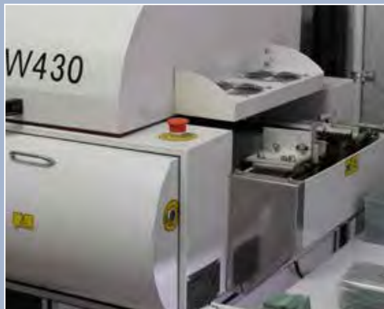
Circuitboard printing equipment
